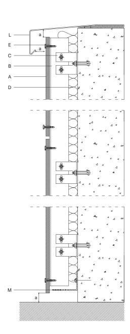
A. Cladding panel B. Vertical metal profile C. Wall bracket D. Insulation E. Screw L. Metal sheet M. Screen a ≥ 20 mm (except for specific technical documents)
