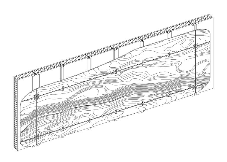
How to install GRCLAD using exposed fastening with screws or rivets
