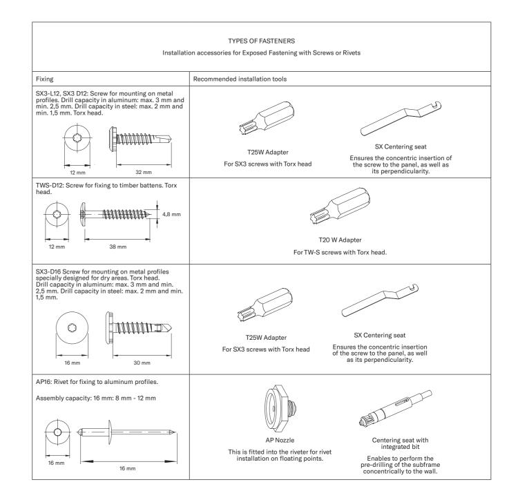
How to install GRCLAD using exposed fastening with screws or rivets
