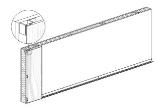
Install the first row of Onesiding clips on the installed plank, using the gauge tool in order to create a 1mm (1/16") expansion joint between the clip and the plank.
