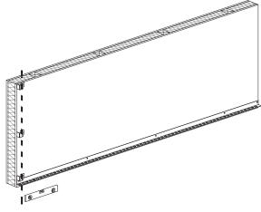
Insert the Onesiding clip tongue into the first plank groove.
