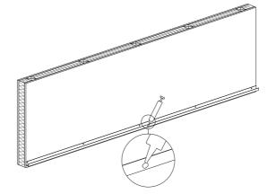
Insert the starter rail tongue into the first plank groove.
