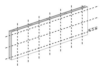
Install the L30X30 Stopper rail at the bottom of the facade fastening it to the supporting wall at a maximum distance of 600mm (24") between fasteners and making sure it is totally plumb. The maximum cantilever distance for the L30X30 Stopper rail is 100mm (4").
