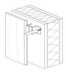
The clips must be installed at least every 600mm (24"). Pieces shorter than 600mm (24") need a third supporting point in the middle.
