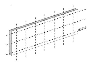
Install the Starter rail at the bottom of the facade fastening it to the supporting wall at a maximum distance of 600 mm (24") between fasteners and making sure it is totally plumb. The maximum cantilever distance for the Starter rail is 100mm (4").
