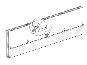
Install the rest of the plank on top of the first following the same process.
