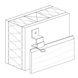
Fastening the Onesiding clips to the supporting element Use the  $\emptyset$  6mm (¼") hole on the Onesiding clip to fasten it to the bearing wall behind. The fastener will depend on the material substrate and it must be provided by others.
