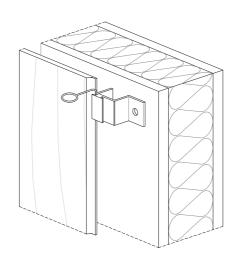
Use the  $\emptyset$  6mm (¼") hole on the Onesiding clip to fasten it to the subframe behind. The fastener will depend on the material substrate and it must be provided by others.
