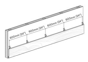
The distance between the Onesiding clips and the edge of the panel must be between 20mm ( $\frac{3}{4}$ ") and 40mm ( $\frac{1}{2}$ ").
