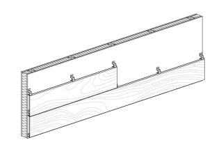
Cut the last plank to finish the facade. Use 1" Jay Shims to shim the facade. Do not use continuous rails to attach the last plank at the top, which may block the airflow behind the panel.
