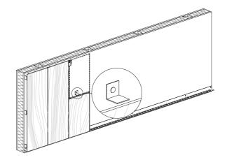
L30X30 Stopper piece. Install the rest of the plank following the same process.
