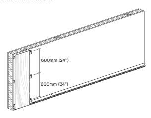
Distances between the Onesiding clips and the edge of the panel. The distance between the Onesiding clips and the edge of the panel must be between 20mm - 40mm (3/4" and  $1\frac{1}{2}$ ").
