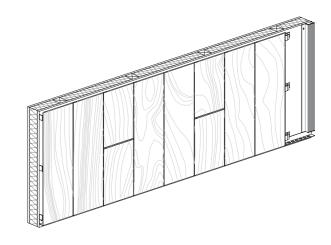
Cut the last plank to finish the facade. Use a continuous Jay to shim the facade.
