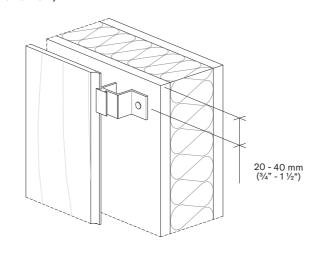
Install the L30X30 stopper piece in the intermediate joints to avoid the plank sliding down.
