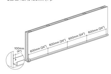
Every plank needs at least one fixed point to avoid pieces moving freely. Add a bit of adhesive for the first plank on the starter rail.
