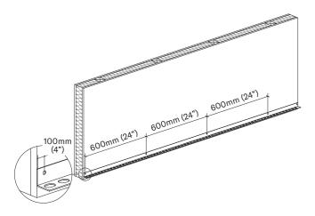
Align the first row of Onesiding clips vertically. The Starter rail supplied for the Horizontal Application can be also used for this step.
