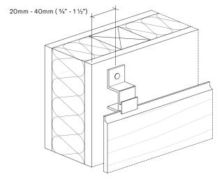
Add a bit of adhesive at least in one of the Onesiding clips per plank to avoid the pieces moving freely.
