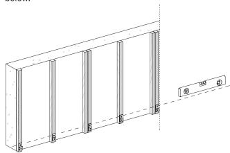
Once the first row of fixing clips has been installed, add the first row of machined planks. The groove in the plank fits into the fixing clip. Once the first row of planks is installed, place the second fixing clip row on the machined edge at the top of the plank. The second fixing clip should be installed upside down, see image below.
