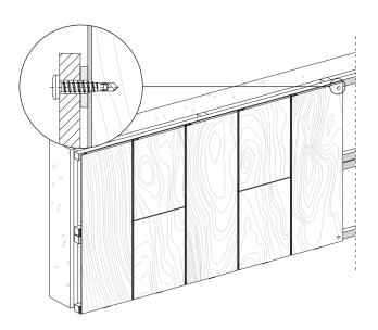
Every plank needs a fixed point to avoid the piece from moving vertically. In order to do so, placing an L20X10 stopper piece below every plank is required. This element creates a fixing point in every piece and avoids them from sliding downwards. Use a DIN 7505B screw to fasten the stopper piece to a wooden subestructure, and a DIN 7504N to fasten it to a metal one.
