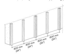
The facade must be installed from the bottom to the top and the subframe must be totally plumb to avoid the panel acquire the imperfection of the facade.
