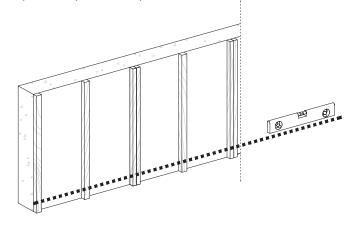
Install the first row of fixing clips at the bottom. The first clip should be placed facing up.
