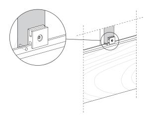
A joint of 6 mm ( $\frac{1}{4}$ ") must be kept between planks placed in the same row. Two fixing clips are necessary to do the joint between panels, so the supporting point behind the joints should be at least 80 mm (3  $\frac{1}{2}$ ") wide.
