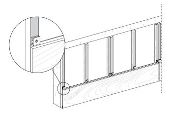
Keep a 1 mm (1/16") distance between the fixing clip and the plank to allow the contraction and expansion of the plank. Use the gap gauge tool for this task.
