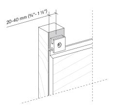
Place the following plank rows one on top of the other. Finally, fix the last row of planks in place using TWS (in case of wooden subframe) or SX3 (in case of metallic subframe) PARKLEX PRODEMA lacquered screws. To ensure the last plank is totally flat, place a 4 mm (5/32") washer behind the top panel or a 4 mm (5/32") thick EPDM tape.
