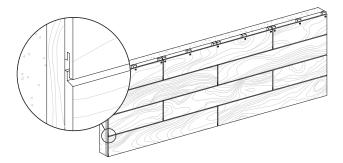
The planks require supporting points every 600 mm (24"). For pieces between 300 to 600 mm (12"-24") a third supporting point in the middle is needed. Pieces shorter than 300 mm (12") only need two supporting points.
