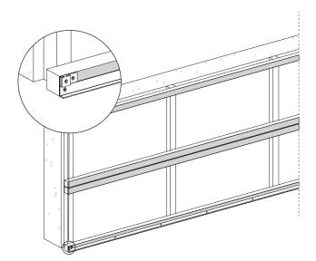
Once the first row of fixing clips has been installed, install the first column of machined planks. The groove in the plank fits into the fixing clip. Once the first column of planks is installed, place the second fixing clip column on the machined edge at the top of the plank. The second fixing clip row should be installed upside down.
