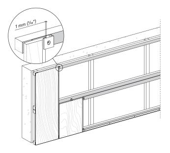
Leave between 20 mm - 40 mm (3/4"-1 1/2") distance from the center of the fixing clip to the edge of the panel.
