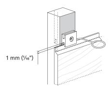
Every plank needs a fixed point, in order to avoid the plank sliding horizontally. In case of wooden subframe use a wooden nail and in case of metal subframe use a BCPA2 screw. This screw or nail should be placed in the center of the plank, so that the expansion/contraction of the material is under control. First, predrill the groove in the center of the plank.
