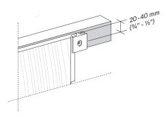
A joint of 6 mm (1/4") must be kept between planks placed in the same row. Two fixing clips are necessary to do the joint between panels, so the supporting point behind the joints should be at least 80 mm (3 1/2") wide.
