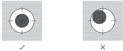
It is also very important for the fixing head to be completely parallel with the panel surface. Be sure that the head of the fastener doesn't make an excessive pressure on the panel and allows its movement due to dilatations. It is recommended the use of a depth locator during installation.
