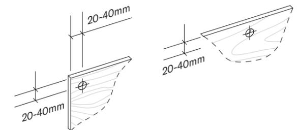
How to install PARKLEX PRODEMA using exposed fastening with screws or rivets
