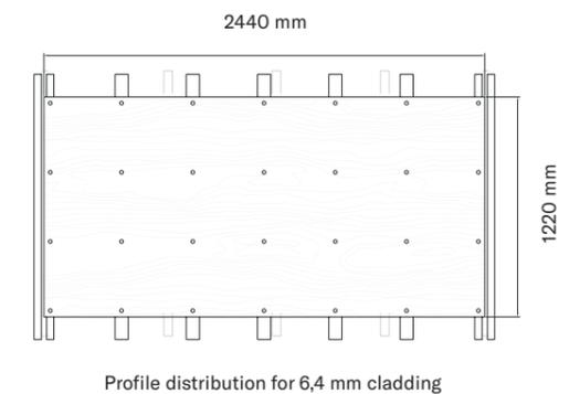
Distance from the edge of the panel to the panel perforation:
