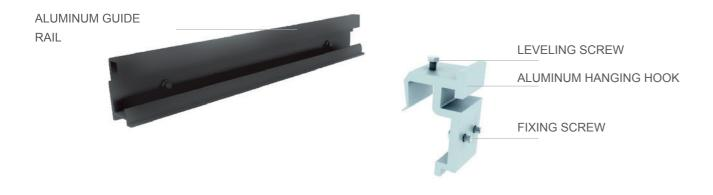
The guide rail are horizontal and mounted over the primary aluminum vertical subframe. Two self-threading screws installed diagonally are used to fasten the guide rail to subframe.
