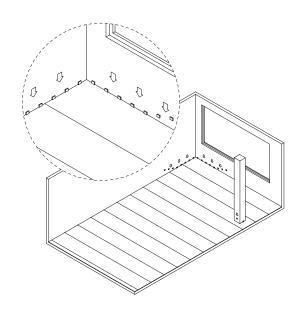
Assemble four pieces with the tongues facing inward toward the herringbone. The apply continuous beads of PVA D3/D4 adhesive to the interior of the upper edge of the groove. This way, the tongue is fully saturated, ensuring a waterproof finish and maximum joint strength.
