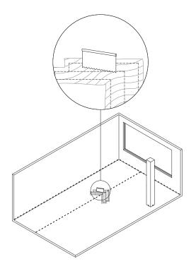
Spread the trowel adhesive to position the next planks one after the other. Repeat the application of PVA D3/D4 adhesive and continue with the installation.
