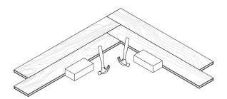
Next, choose the position of the herringbone based on the desired design. Then, place a string line along the room to maintain alignment throughout the installation.
