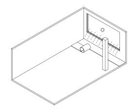
During the installation process, place temporary wedges of  $\geq$  8mm around the perimeter, next to the walls or other fixed points, to allow for future expansion/contraction.
