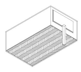
After 24 hours, remove the temporary spacers from the perimeter and install a baseboard of adequate thickness to cover the perimeter joints.
