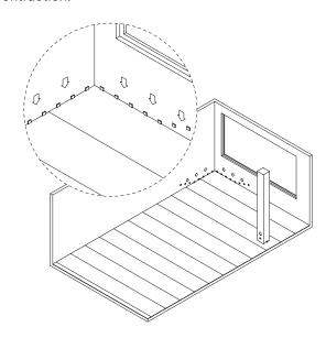
Four pieces are assembled with the tongues facing inward toward the herringbone. Continuous beads of PVA D3/D4 adhesive are then applied to the interior of the upper edge of the groove.
