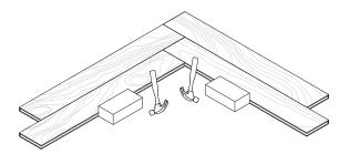
Next, choose the position of the herringbone pattern based on the desired design. Then, place a string line along the room to maintain alignment throughout the installation.
