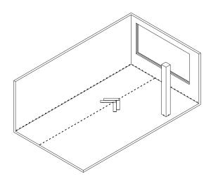
Once the first pieces are assembled, spread the gluing down adhesive on the subfloor. Align one of the tips with the string, and apply the gluing down adhesive where the first planks will be placed.
